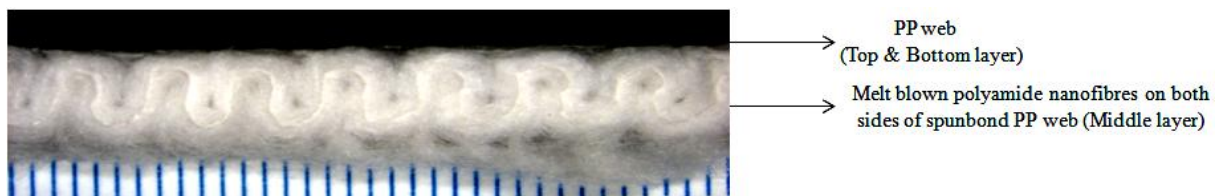
Figure 9. Needle punched struto nonwoven structure.
