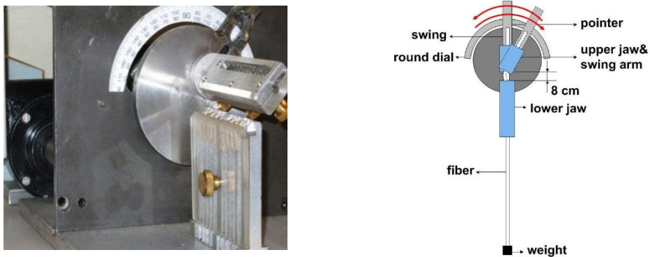
Figure 4.3 Prototype device to measure resistance to bending (left) and corresponding schematic diagram of side view (right).
