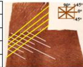
Figure 9. Barkcloth Fabric Reinforced Composite (BFRP) Laminate layering sequence
