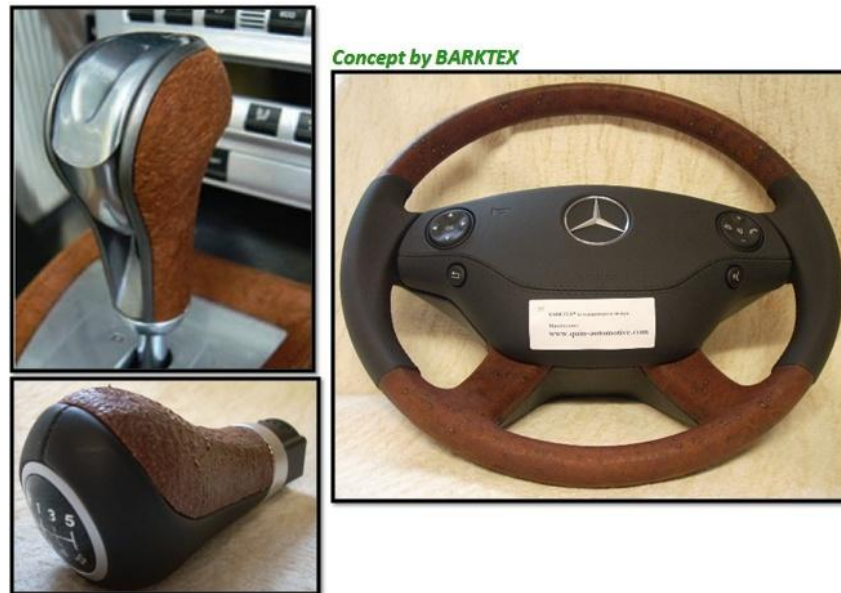
Figure 34. Barkcloth fabric and reinforced composite automotive applications. (Image courtesy of Barktex)
