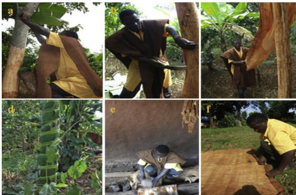
Figure 2. Extraction of Barkcloth non-woven natural fabric: (a) Scrapping of tree outer layer. (b) Use of local wedged tool to peel off the bark. (c) Peeling of the bark. (d) Covering of the tree stem for environmental sustainability. (e) Pummeling under the shade. (f) Sun drying of the non-woven fabric. [25]
