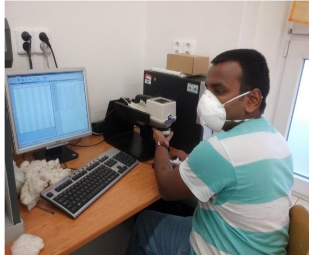
Figure 2. Miniscan XE (spectrophotometer) used for the Spectral data as well as CIE XYZ values in the LCAM at Technical University of Liberec.
