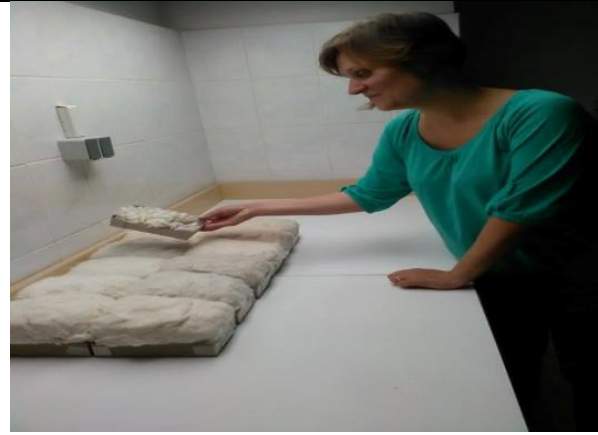
Figure 7. Visual assessment of Pakistani cotton with white background by taking USDA cotton as reference standard.
