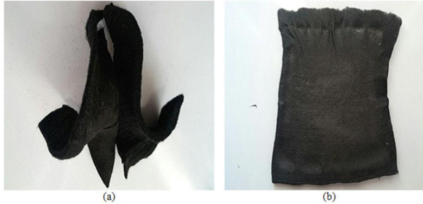
Figure 10. Activated carbon from stabilization (a) without any pre-tension, (b) with applied pre-tension
