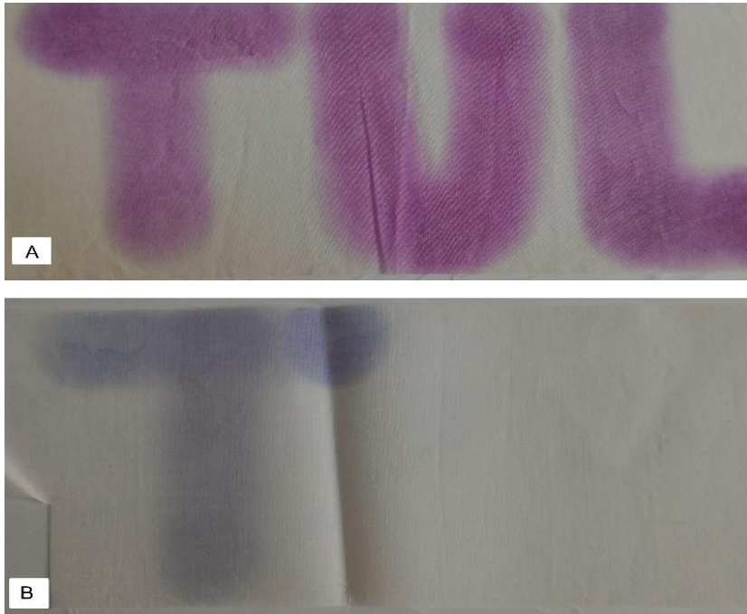
Figure 18: Photochromic sol-gel coated fabric, (A) fabric coated with APS precursor and (B) fabric coated with OTES precursor (Colored portion indicates the influence of UV radiation).
