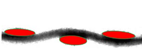
Figure 18. Elliptical substitution of the yarn cross-sectional shape in the cross-section of woven fabric
