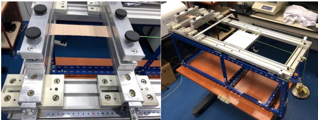
Figure 10. The experimental design and testing of manual tensile testing device
