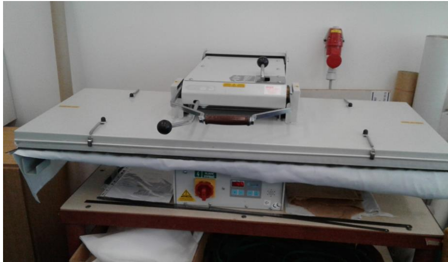
Figure 1. Lamination by Comel PL/T 1250 Heat and Press Machine.
