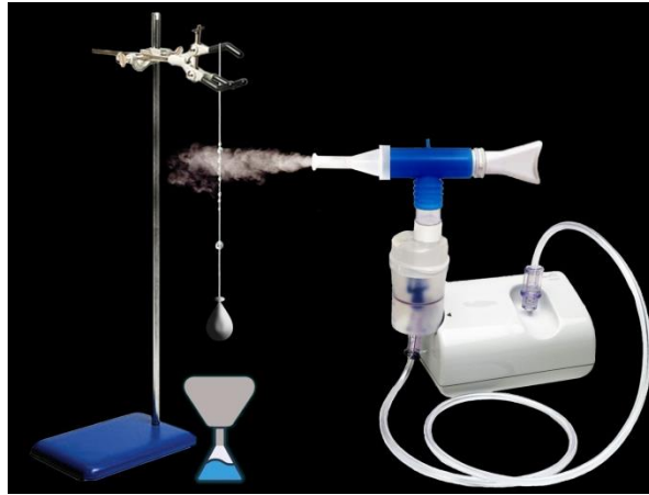
Figure 9. The diagram of the experimental setup for fog collection.
