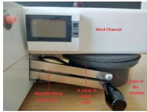
c. Showing outer rings were stacked on the base of the hotplate
