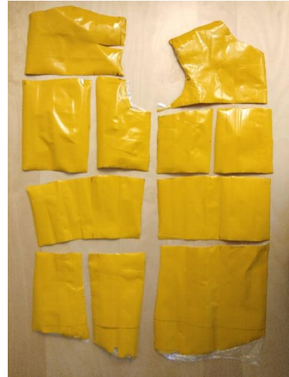
c. Unmolded front and back pieces and were divided into small segments according to the contour lines on the manikin's torso
