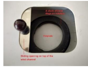
d. Showing inner rings were placed inside the wind channel on the hotplate
