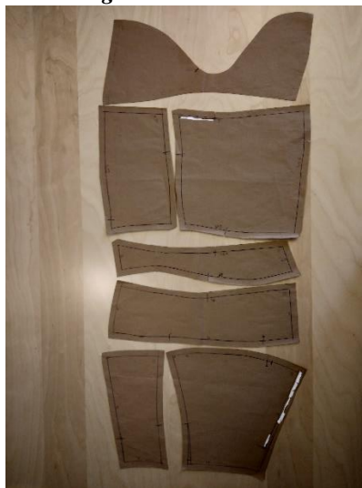
e. The arm piece was converted into two-dimensional sleeve patterns
