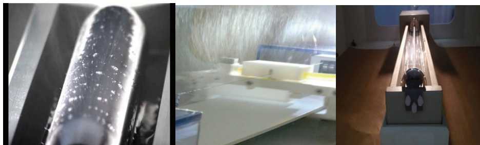
Figure 1 Rotating roller electrode, Single wire electrode and Rotating wire electrode (from left to right)
