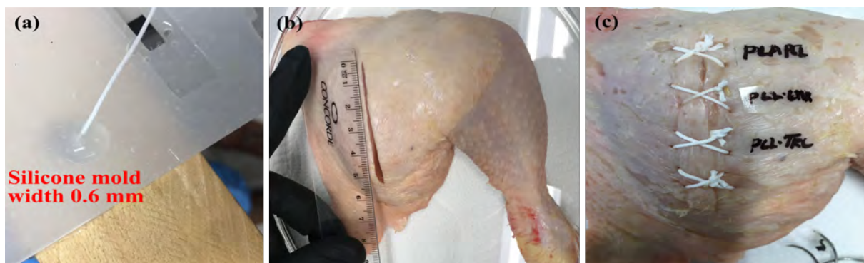
Figure 2.4: (a) Setup of the abrasion experiment using silicone mold with PBS, (b) incision of chicken thigh, and (c) stitched incision using various resultant braided yarns.
