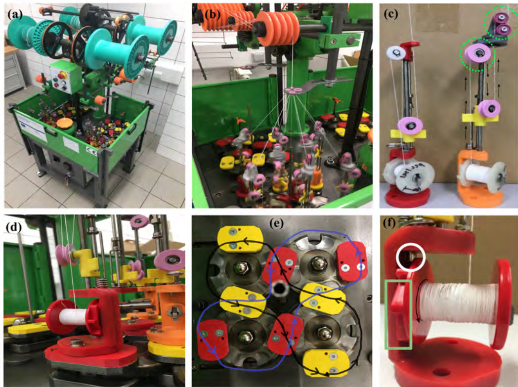
Figure 2.2: Images of the braiding machine and its components. (a) The braiding machine, (b) a close-up view of the yarn braiding process, (c) commercial yarn carriers (left) and custom-built yarn carriers (right, green circle highlights the modifications), (d) horn dog with a carrier, (e) arrangement of horn gears (black and blue lines indicate the path of the horn dog with the carrier), and (f) pawl (circle) and ratchet (rectangle).
