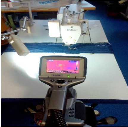
Figure 3 Thermal camera FLIR P60 with Lockstitch machine
