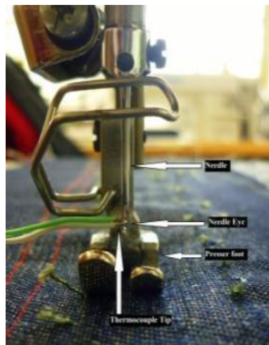
Figure 2 Thermocouple placement for thermocouple touch method
